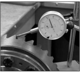
the pinion. If I want to increase the backlash by 0.007" I move the ring gear 0.010" farther away from the pinion. This is not exact for all ring & pinion sets, but it is a good general guideline.
